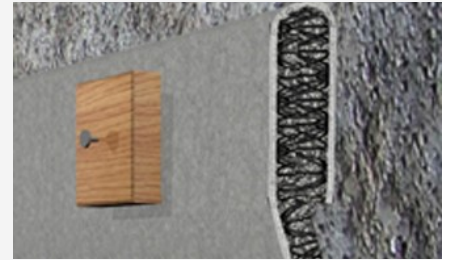
On top of the wall, EnkaDrain is folded up on itself, no need of special accessories.
